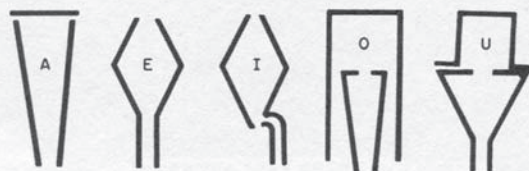
FIG. 9. Kratzenstein's resonators for synthesis of vowel sounds. The resonators are actuated by blowing through a free, vibrating reed into the lower end. The i sound is produced simply by blowing into the lower pipe without a reed. 1
